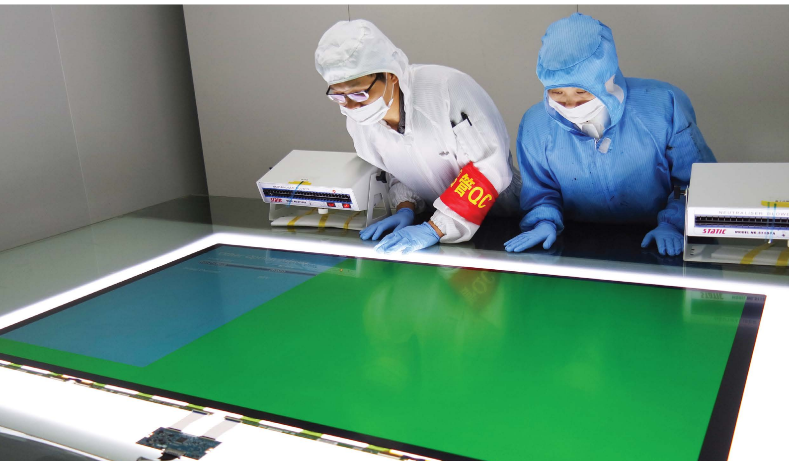
Inspection of an 86" optically bonded display screen
