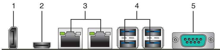
1. **DisplayPort connector.** This port connects a device with DisplayPort connector.
